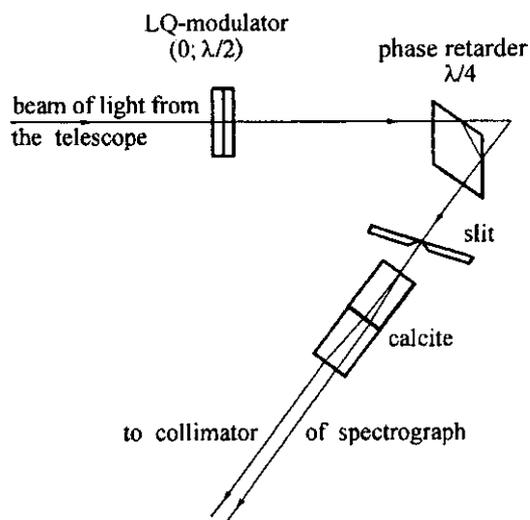
Figure 3: *The schematic diagram for measurements with the BTA MSS.*
